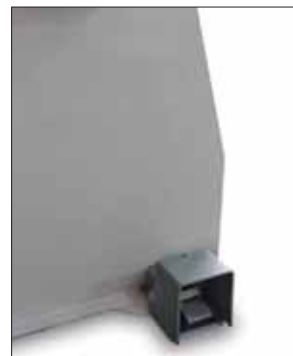
The interlocked cover and a separate foot pedal ensure maximum operation safety.
