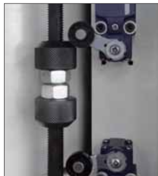
Modified actuators enable fine stroke adjustment.
