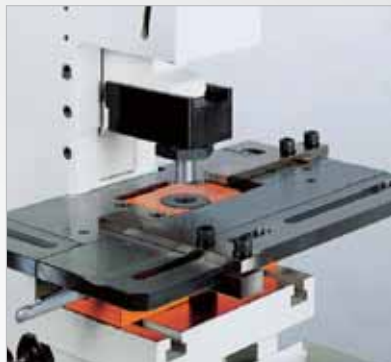
*Punching tool on notching station.
